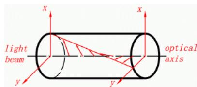
The plane of polarization of linearly polarized light will be rotated by Quartz Crystal due to the optical activity. Eastoptics's polarization rotators have very high temperature bandwidth and can be easily used in rotating the polarization of lasers.
