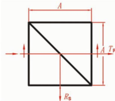
Polarization Beamsplitter Cubes are constructed by cementing two precision right angle prisms together with the appropriate interference coating on the hypotenuse surface. The P-polarization of the input beam is transmitted, and S-polarization of the input beam is reflected.
