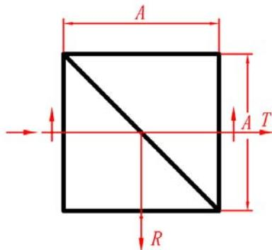
Beamsplitter Cube is a more sophisticated type consisting of two right- angle prisms cemented together at their hypotenuse faces. The cemented face of one prism is coated. Before cementing, with a metallic or dielectric layer having the desired reflecting properties, both in the percentage of reflection and the desired color. The absorption loss to the coating is minimal and transmission and reflection approach 50%.
