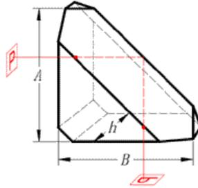
Amici prisms, also called "Roof prisms" or "Right angle roof prisms" revert and invert the image as well as bend the line of sight through a 90° angle. Ideal for use in spotting scopes, and any optical instrument where it is desirable to take an inverted image from an objective, turn it right side up, and bend it through a 90° angle in order to maintain the correct visual orientation.
