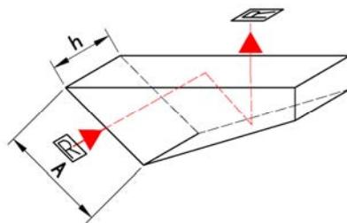
Half Penta Prism is used to deflect a straight light 135 degree, it is exactly an half cut from penta prism, it is widely used in telescope systems.
